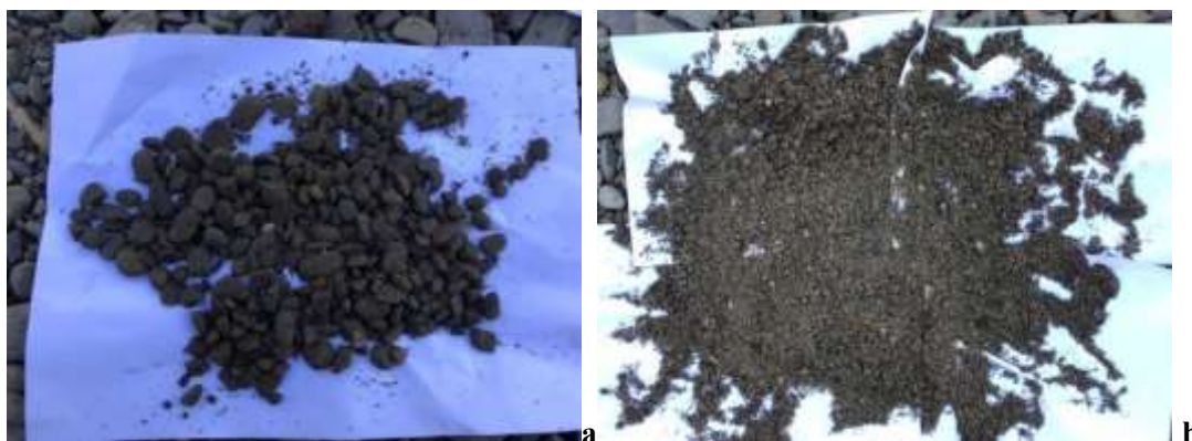
Figure 10. Well-rounded fragments: a - size 10-2 mm of the first series of samples; b - size less than 2 mm of the first series of samples (author – Mykhailo Mykyta, date – 22/06/2024)
