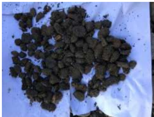
Figure 9. Sandstone with a size of 40-10 mm in the second sample (author – Mykhailo Mykyta, date – 22/06/2024)
