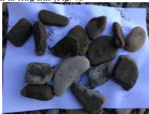
Figure 4. Debris larger than 40 mm in the first sample (author – Mykhailo Mykyta, date – 21/06/2024)
