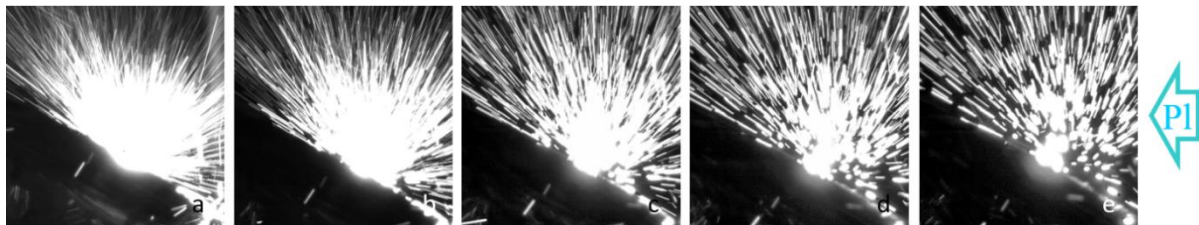
Fig. 2. Images of PSI after a plasma impact on an inclined CPS target (with an incoming plasma energy density of 3 \text{ MJ m}^{-2} ). The images correspond to 1.2-2.4 ms (a); 2.4-3.6 ms (b); 3.6-4.8 ms (c); 4.8-6 ms (d); 6-7.2 ms (e) after the start of the PSI ( t_{\text{exposure}}=1.2 \text{ ms} )
