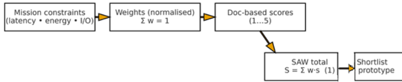
Fig. 1. Selection workflow from qualitative criteria to prototype shortlisting (SAW)
