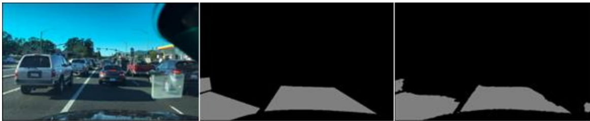
Fig. 2. An example of the input image of the test subset (left), the true mask (middle) and the predicted mask (right) with the EfficientNetV2_s model.
