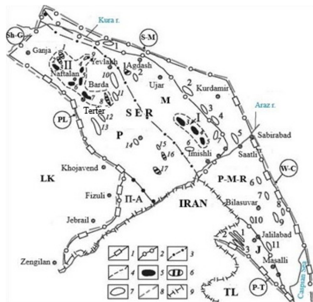
Fig. 7. Scheme of tectonic and oil-gas-geological zoning of the Yevlakh-Agjabedi oil and gas region (OGR) and the Pre-Talysh-Mingachevir low-prospect region Middle Kura-Kartli oil and gas subprovince (NGSP) of the Transcaucasian oil and gas provinces (NGP)
