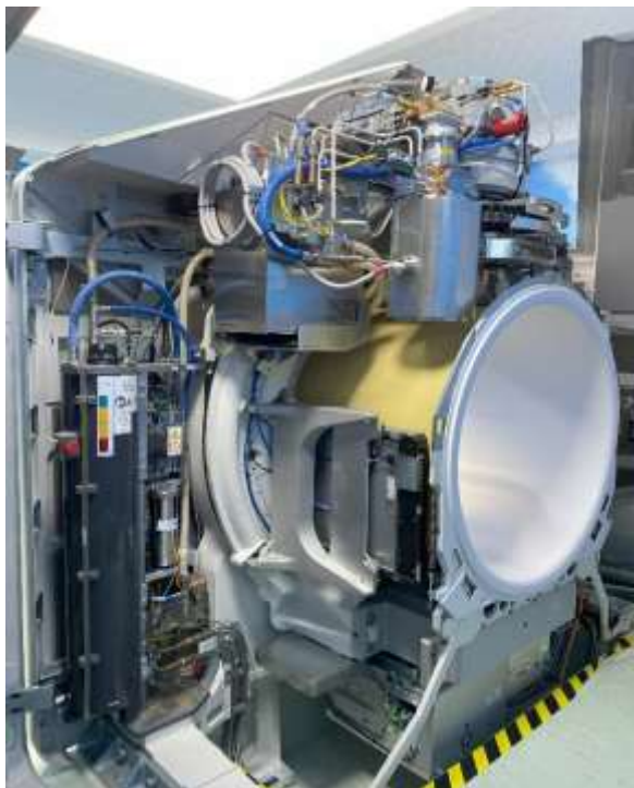
Fig. 1. O-ring linear accelerator Halcyon - view under the covers
