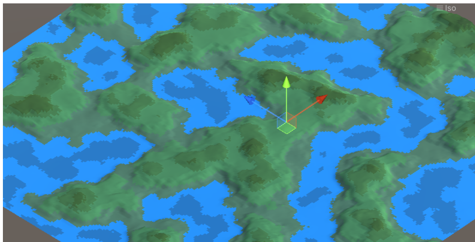
Рисунок 2.18 – Болото. scale=62 , octaves=3 , persistence=0.29 , lacunarity=3.0 , multiplier=150 , erosionSteps=2 , erosionLimit=0.06
