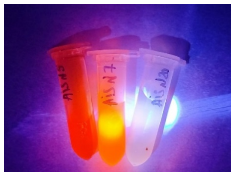
Fig.1 Photo of Ag-In-S colloidal solutions with various molar ratio under laser excitation at 406 nm
