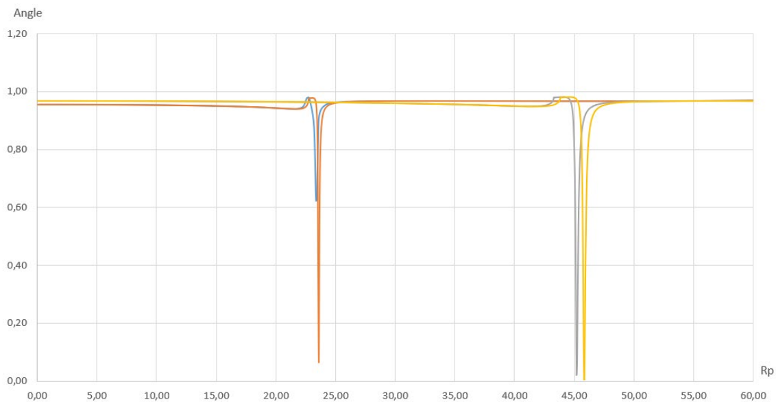
Figure 2. The graph of the dependence of the angle of incidence for two types of material on the change in the refractive index
