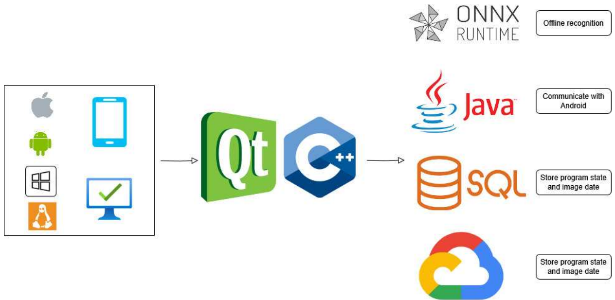
Figure 6.3: Upper-level architecture of the app
