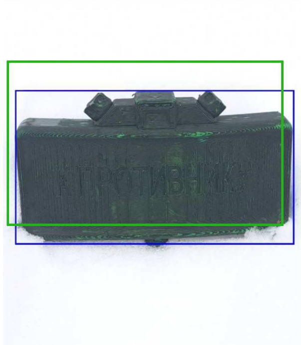
Figure 2.7: Ground truth (blue) and predicted (green) bounding boxes. IoU is calculated from their intersection and union areas
